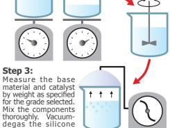
mixture to remove air that became entrapped during mixing. The mixture will rise while degassing, and therefore, a container of adequate size (4 to 5 times) is required.
