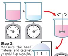
Measure the base material and catalyst by weight as specified for the grade selected. Mix the components thoroughly. Vacuum-degas the silicone mixture to remove air
