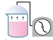
Vacuum-degas the silicone mixture to remove air that became entrapped during mixing. The mixture will rise while degassing, and therefore, a container with of adequate size (4 to 5 times) is required.
