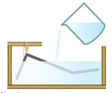
Begin pouring the matereial, starting first at a low point in the mold. It is advisable to and supporting structure. Remove any flash vacuum degas once again after pouring, as that may have developed along the edges. some air will enter the silicone while pouring. Allow the silicone to cure for the specified time and conditions
